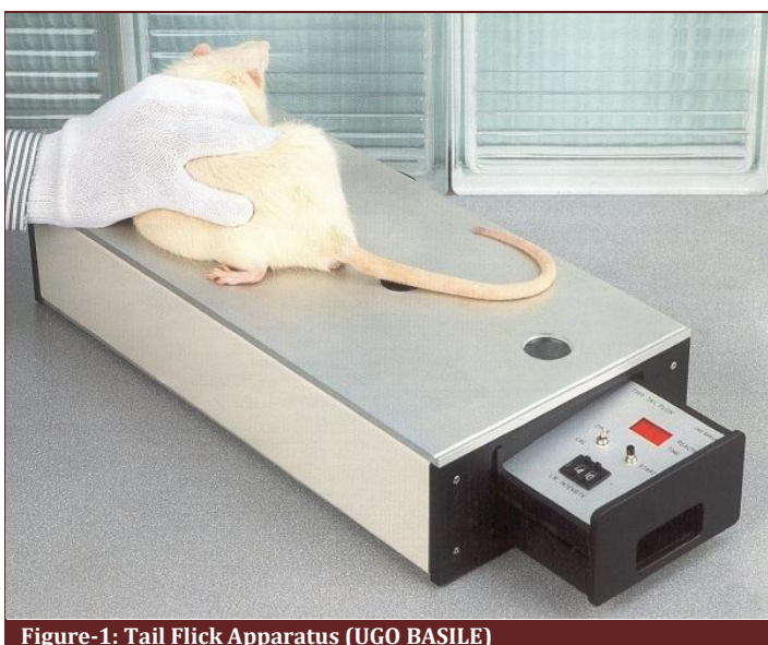
Figure-1: Tail Flick Apparatus (UGO BASILE)
